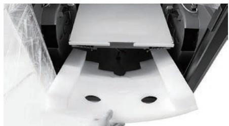
6. Press and hold [Z-] continuously until the build plate rises to a higher position, and then take out the foam block below.
