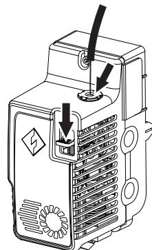
4. Insert the filament into the filament feeding inlet continuously until the filament goes through the filament guide tube.
