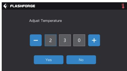
8. Filament feeding operation: Click the [Tools]-[Filament] button on the screen in turn, and set a reasonable heating temperature according to the required temperature value of the material; Operate according to the screen prompts, and wait for the nozzle to extrude uniform filament smoothly.
