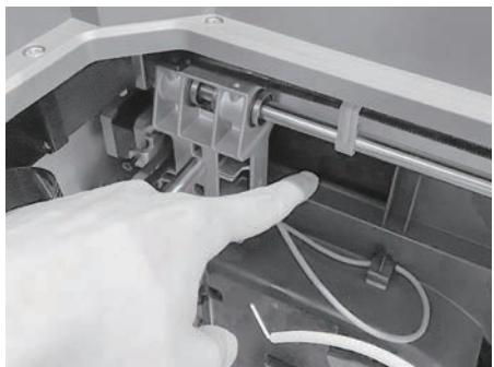
4. Remove the buckles on the X-axis and Y-axis synchronous belts.
