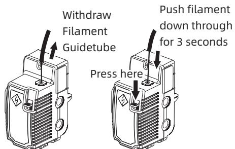
Filament unloading operation: Click [Unload], press down the filament pressing plate after the extruder temperature heating is completed, pull out the white filament guide tube, and pull out the filament upward quickly and then filament unloading is completed.
