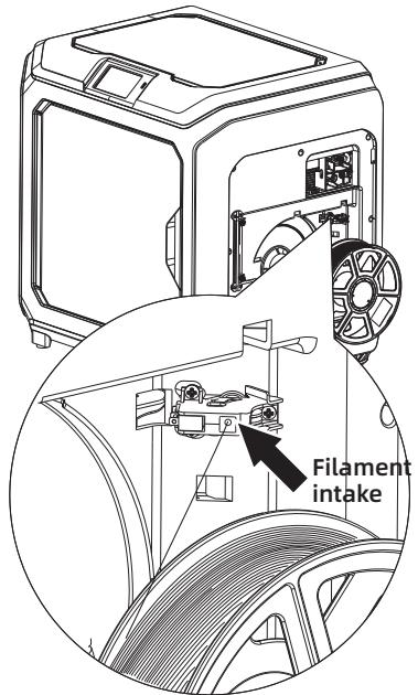
2. Take out the filament and insert it into the filament feeding inlet.
