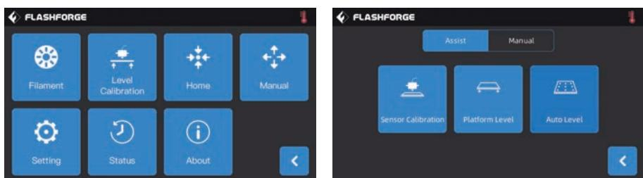
9-point leveling function: when the printing flatness is still poor after the platform leveling and XY/Z axis calibration, this function can be used to compensate for better flatness;
