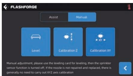
Manual leveling mode: Execute platform leveling, Z-axis calibration and X, Y axis calibration in turn. This is a complete set of leveling and calibration operation procedures.
