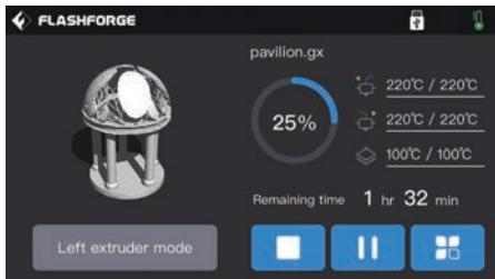
5. The printer starts to heat up and will start printing after heating completed.
